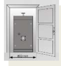
Outer shell with oval shape. Models up to 630 kW can pass through a 800 mm wide door.
